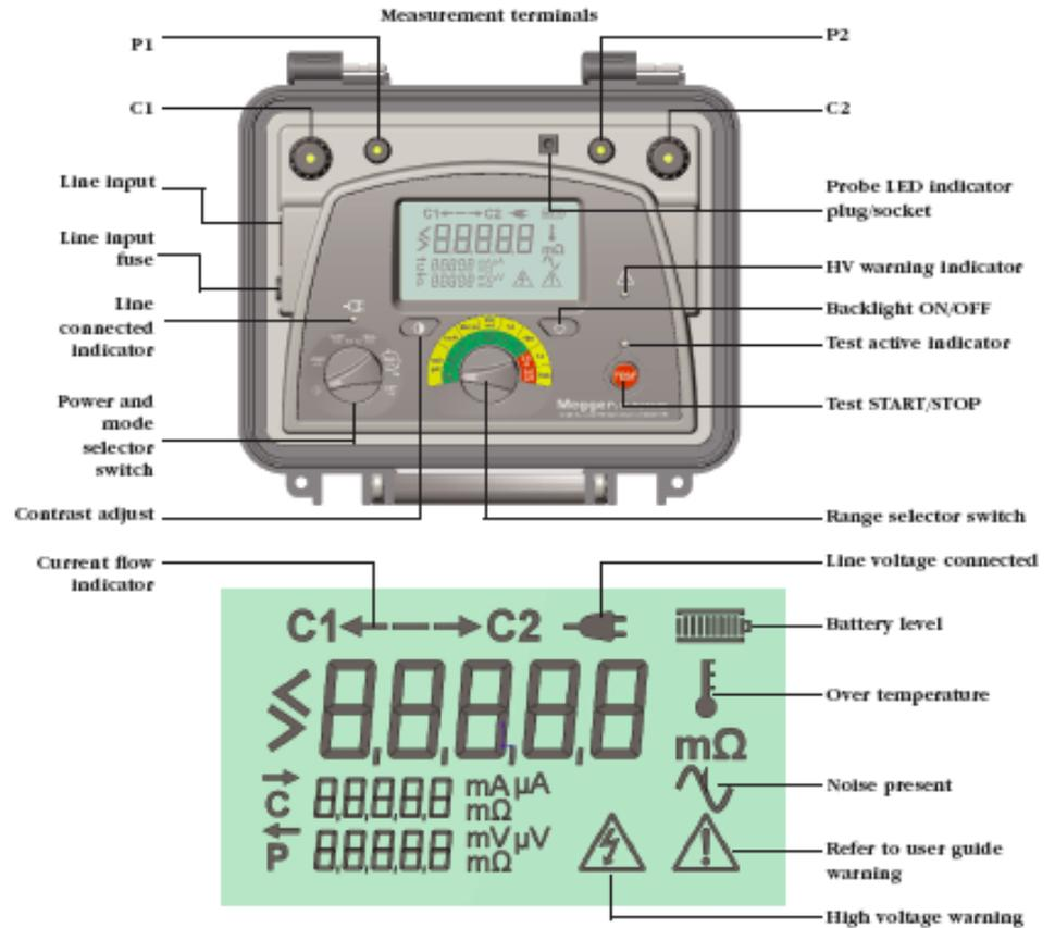
After starting a test the user will see confirmation of successful continuity testing on the LCD. If the dashes are not shown connecting 1 & 2 C and/or P leads connection has not been detected.
